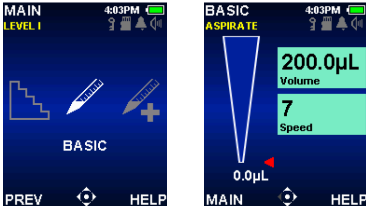
Figure 8: Basic Mode Highlighted in Level I Menu (left), Basic Mode Operating Screen (right).
