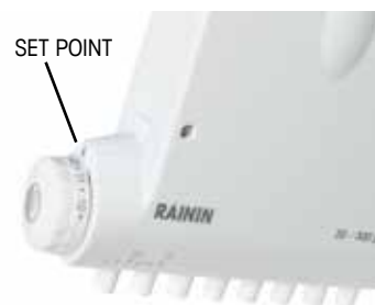
Figure 37: Limiter Set Point
