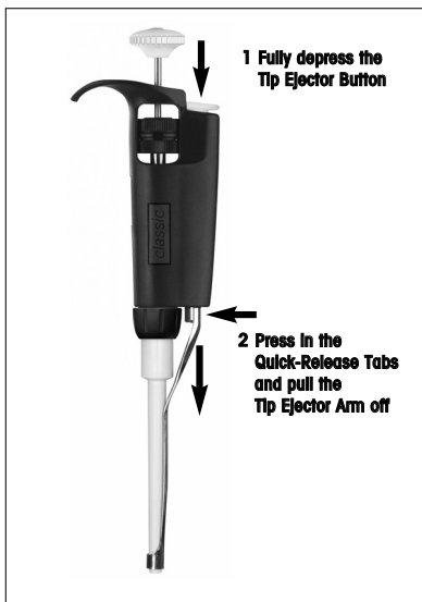
Figure 3 Removing the Tip Ejector Arm
